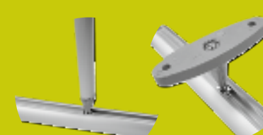
Anchoring on profile rail: possible along the whole length by means of square nut; for adjustable ceiling mount RVS/DS or with ceiling bracket RVS/DH. Max. spacing: 2 m.
